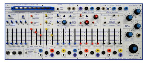
Set the knobs, sliders, and switches on the music easel to their default shipping settings, as shown above. Connect the main audio output (side of case) to your sound system or plug headphones into the Easel's frontpanel headphone jack.
