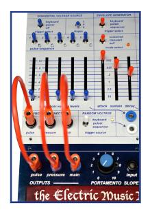
Using three of the included banana jack cables, connect the Pulse, Pressure, and Main CV outputs at the top left of the keyboard to the corresponding Pulse, Pressure, and Pitch CV inputs at the lower left of the 208. Then set the
