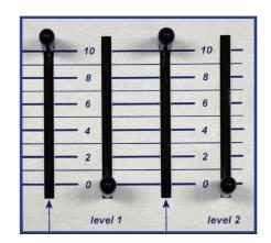
Lower the Level 1 and Level 2 sliders to their minimum positions (0) and raise the corresponding Level 1 and 2 CV input sliders to their maximum (10). The Dual Lo Pass Gate will now open and close entirely in response to the Control Voltages from the Envelope Generator. Play some notes on the keyboard to audition your handiwork.
