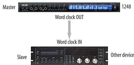
Figure 4-11: Slaving another digital audio device to your MOTU device (a 1248 in this example) via word clock. For the 1248 clock source, choose any source besides word clock, as it is not advisable to chain word clock.
