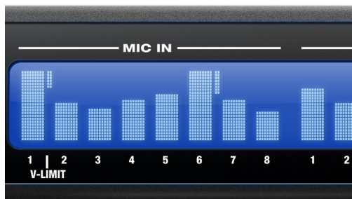
Figure 6-1: V-Limit compressor on the 8M interface.
