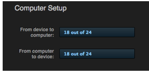
Figure 3: The 'From device to computer' setting determines how many channels you see in the Left Input and Right Input menus.
